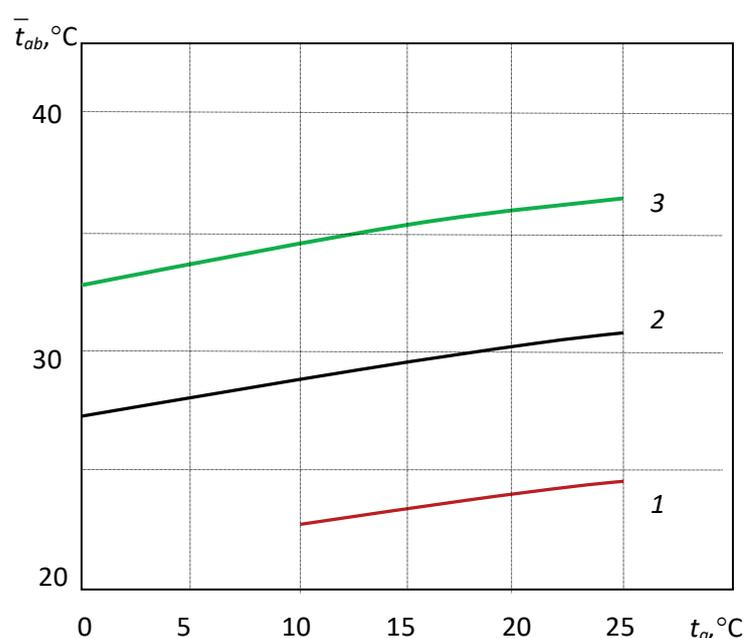
FIGURE 4. Dependence of temperature of an absorber on ambient temperature and irradiance at the variable consumption of a fluid, W/m<sup>2</sup>: 1 - 200; 2 - 500; 3 - 800
