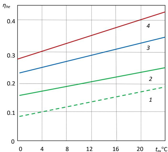
FIGURE 3. Influence of external conditions on heat transport efficiency ratio at the constant charge of a fluid. Length of the channel, intensity of radiation: 1 - 1 m, 500 W/m<sup>2</sup>; 2 - 1 m, 800 W/m<sup>2</sup>; 3 - 1.5 m, 800 W/m<sup>2</sup>; 4 - 2.0 m, 800 W/m<sup>2</sup>
