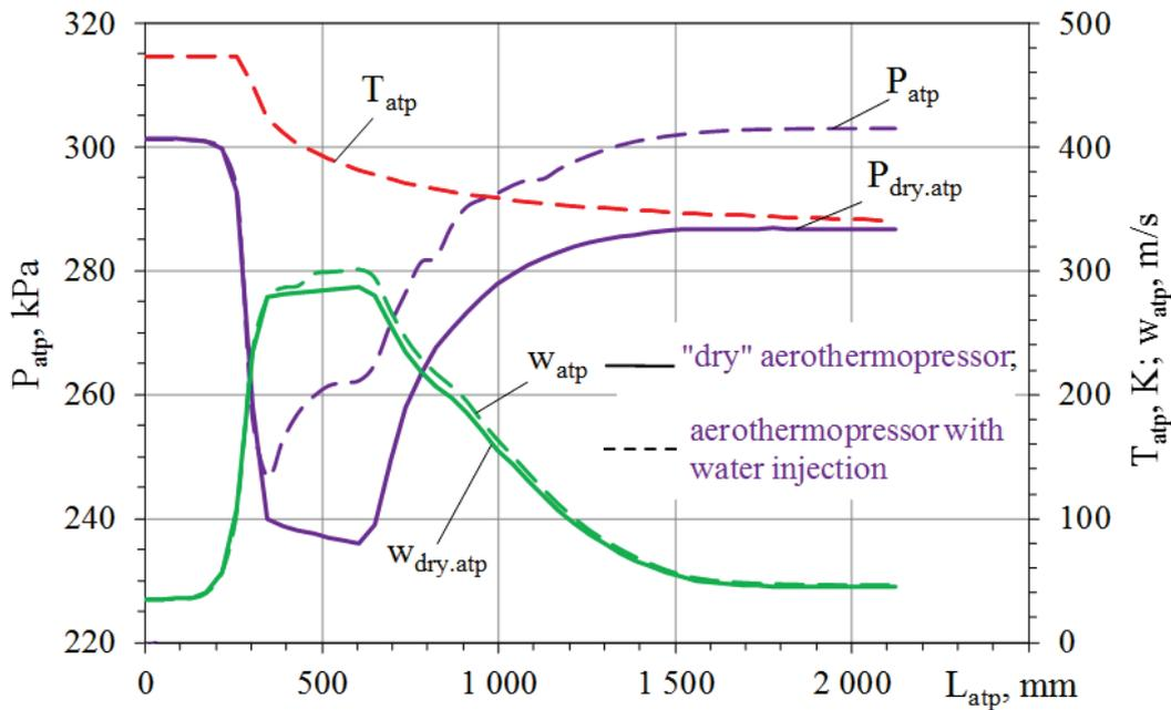
**FIGURE 2.** Dependences of the flow main characteristics: total pressure  $P_{atp}$ , flow velocity  $w_{atp}$ , flow temperature  $T_{atp}$  on the length of the aerothermopressor flow part  $L_{atp}$
