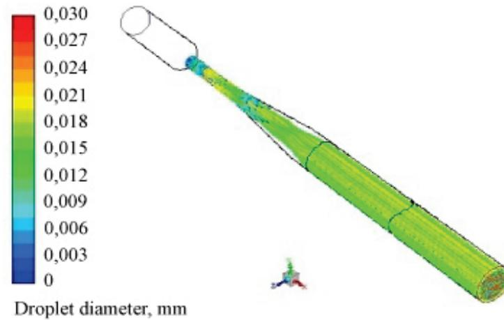
**FIGURE 3.** Dispersion distribution of sprayed water  $\delta_p$  in the flow path of the aerothermopressor for incomplete evaporation, with obtaining smaller droplets at the outlet of the diffuser part of the apparatus ( $g_w = 10\%$ )
