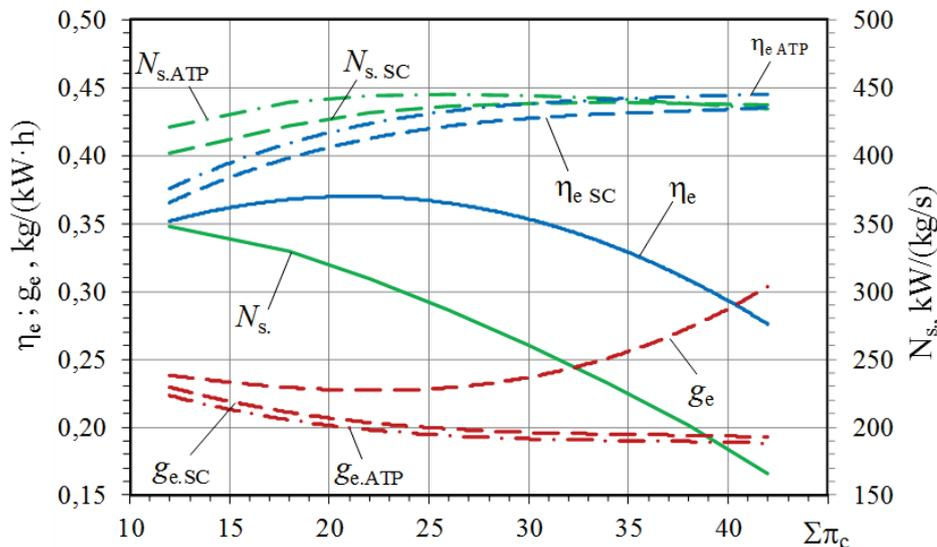
**FIGURE 5.** Dependences of specific power output ( $N_s$ ), specific fuel consumption ( $g_e$ ) and efficiency ( $\eta_e$ ) on the total compression ratio ( $\Sigma\pi_c$ ) in compressors for the simple cycle, the complex cycle with a surface air cooler (SC) and the complex cycle with an aerothermopressor (ATP)
