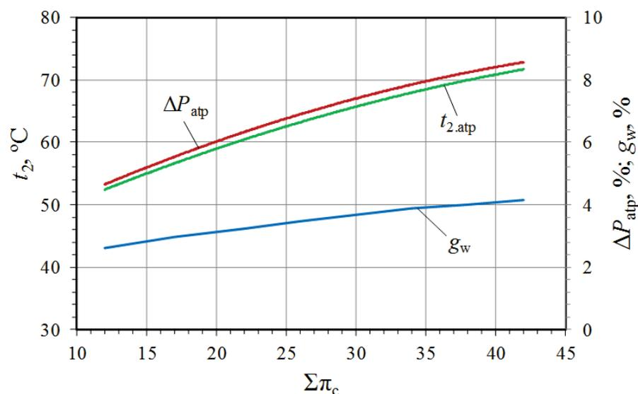
**FIGURE 4.** Dependences of the outlet air temperature ( $t_{2.atp}$ ), the relative water flow rate ( $g_w$ ) and the relative pressure increase at the aerothermopressor outlet ( $\Delta P_{atp}$ ) on the total compressor pressure increase  $\Sigma\pi_c$
