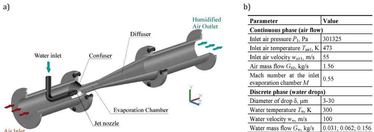
FIGURE 1. 3D model of the aerothermopressor (a) and the main inlet parameters of the airflow and water injection (b)
