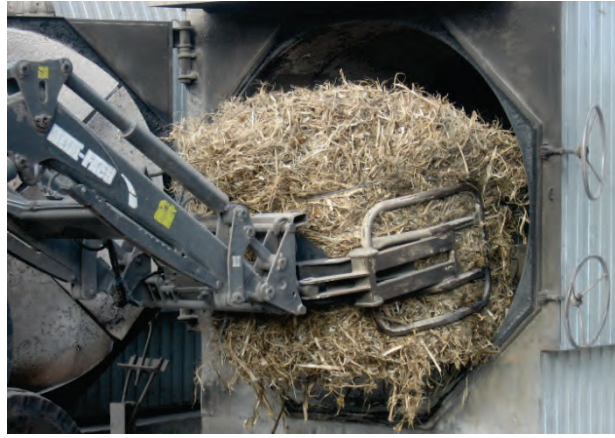
Figure 3. Loading a bale of crushed sunflower stalks into the heat generator of the grain dryer.
