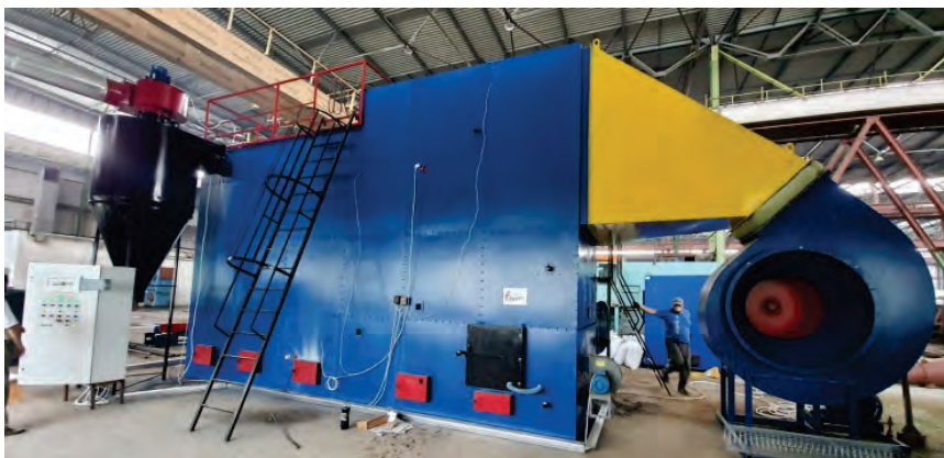
Figure 1. Exploratory prototype of a 2500 kW heat generator-utilizer with the principle of vortex combustion of uncertified fuel.
