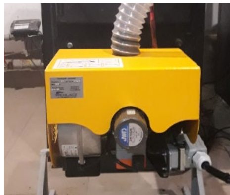
FIGURE 4. Automatic burner with a movable scraper
