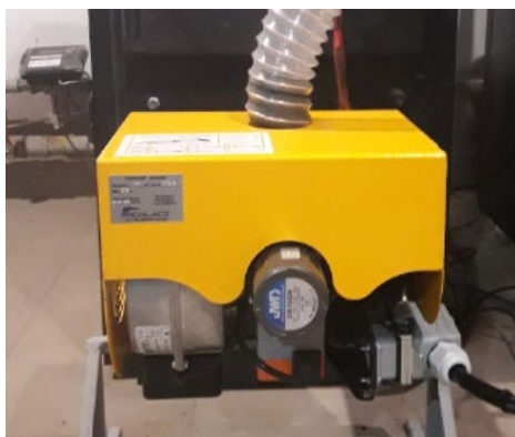
FIGURE 4. Automatic burner with a movable scraper
