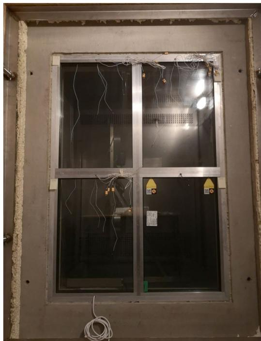
**FIGURE 2.** Photograph of the climatic chamber testing plane
