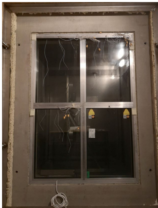
FIGURE 2. Photograph of the climatic chamber testing plane
