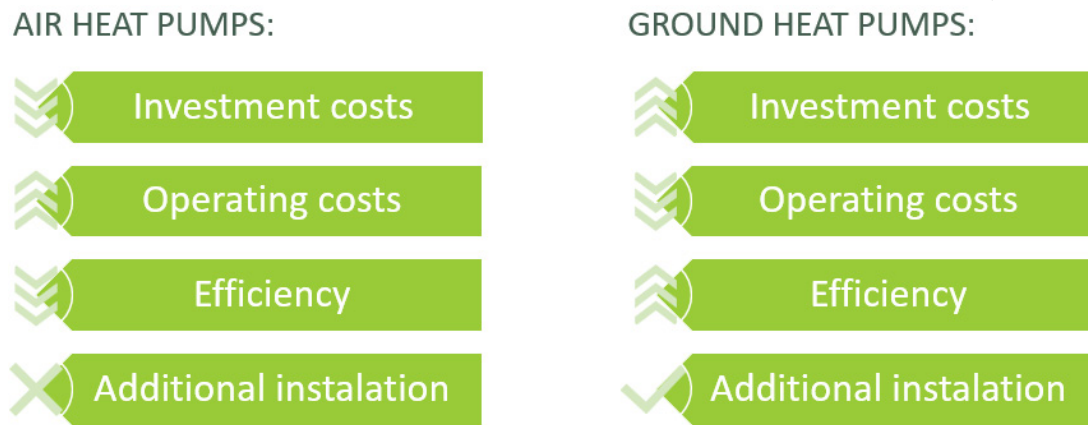
Figure 5. Comparison between air and ground heat pumps
