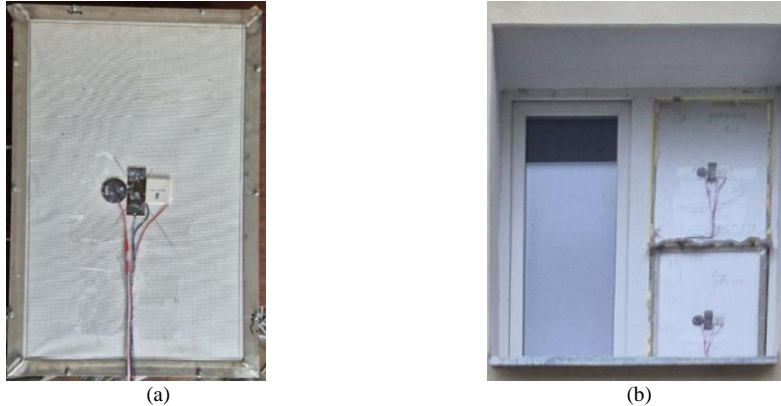
Figure 1. Vacuum insulation panels. (a) used in experimental study with installed heat flux density and temperature sensors; (b) mounted in a window frame for field testing
